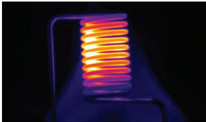
Images through standard glass for high temperature measurements
